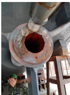
Figure 2. Vessel 3 (PTSC 05 tugboat) after 5 years, Nghi Son port: bearing bore - moderate uniform wear; AISI 421 shaft - no abrasive damage
