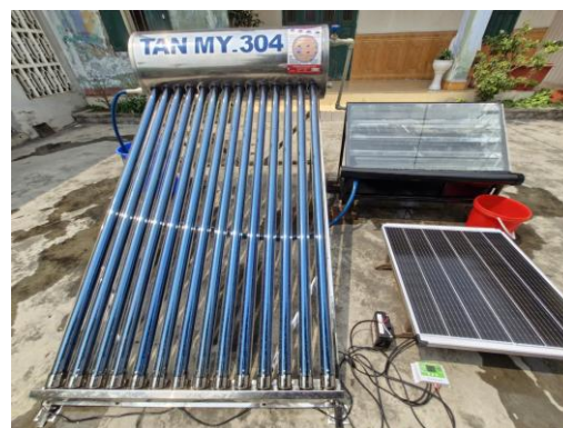
Figure 1. A solar water distillation system integrated with an evacuated tube collector and a stepped evaporation chamber
